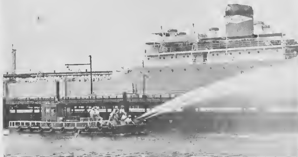
CREW MEMBERS put the new craft through its paces as they approach a dock under full power with turrets throwing salt water under full pressure. The low-built turrets are excellent for fighting fires under the docks.
